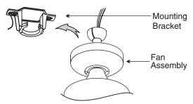
Rotate the fan so that the groove on the ball engages the ridge on the mounting bracket.
