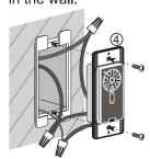
⑤ Position and install the wall cover plate with the wall plate screws.
